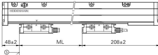
The shipping brace already sets the proper gap between the scale-tape housing and the scanning unit.
