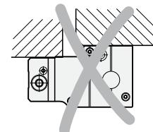
If there is an increased risk of contamination, mounting an additional cover with seal between the mounting surface and the cover is recommended.
