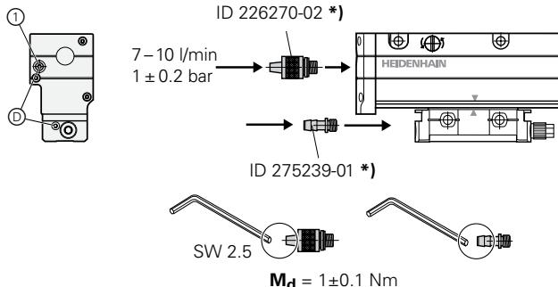
Connection of compressed air via connecting piece **with** throttle function
