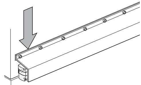
Ensure that the mounting surfaces is free of paint, dust or grease!
