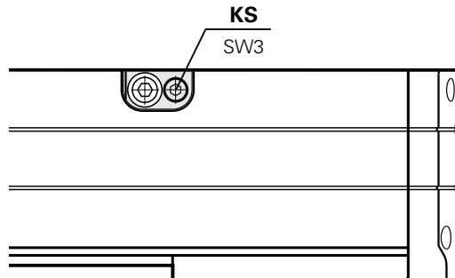
Release clamping screw **KS** with about 2 revolutions.
