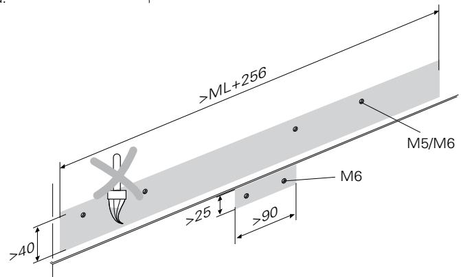
Choose a mounting attitude such that the maximum traverse range is within the measuring length ML of the encoder.
