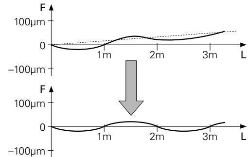
Set up a comparator system (such as a laser interferometer) in the workpiece plane and measure the machine.
