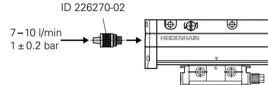
Connection of compressed air via connecting piece **without** throttle function
