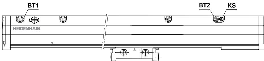
**KS** clamping screw fixed: Same thermal behavior as machine base (Mounting option 1).
