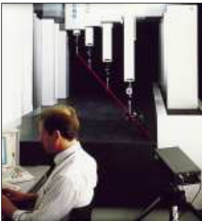
CMM space-diagonal calibration using laser measurement system.
