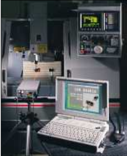
Machine tool calibration of linear axis using laser measurement system.
