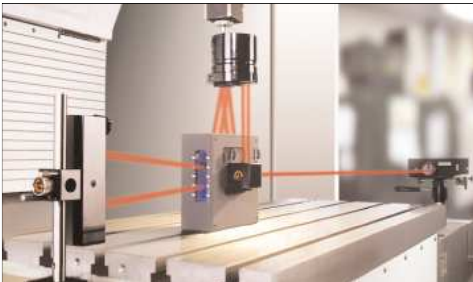
X-Z axis squareness measurement on a VMC
