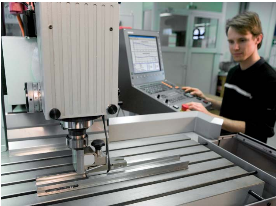
Determining the positioning accuracy with a VM 182
