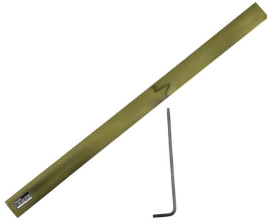
Visible marking on the test film after contact with an Allen wrench, as an indicator of tool magnetization
