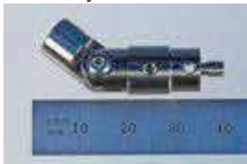
M4 rotary knuckle with ball bearing for unlimited radial adjustment and a clevis knuckle for 180 degree axial adjustment. Stainless steel. Overall length is 33.0 mm.
