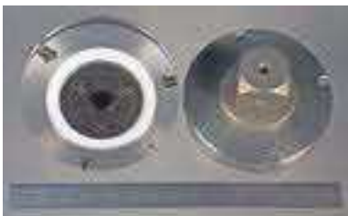
M5 adapter plate for VAST-XT probe system with hard anodized aluminum cube. 69.0 mm diameter.
