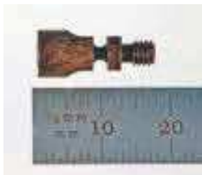
"Weak Link" with M4 male and M4 female threads. Machined from SAE 4140 chromoly steel. Black oxide finish.
