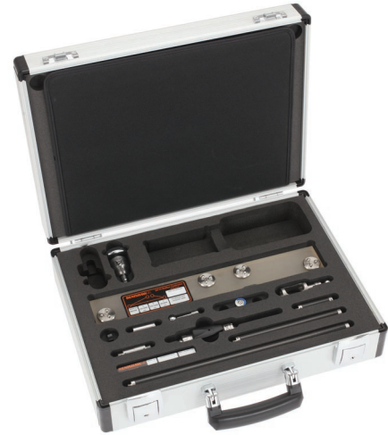
QC20-W ballbar kit with Zerodur® calibrator
