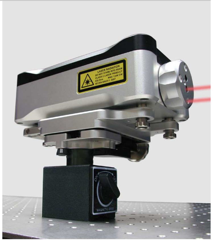
XL-80 laser mounted on a magnetic base
